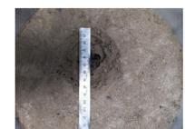
Figure2: Significant erosion in CEF7 core
