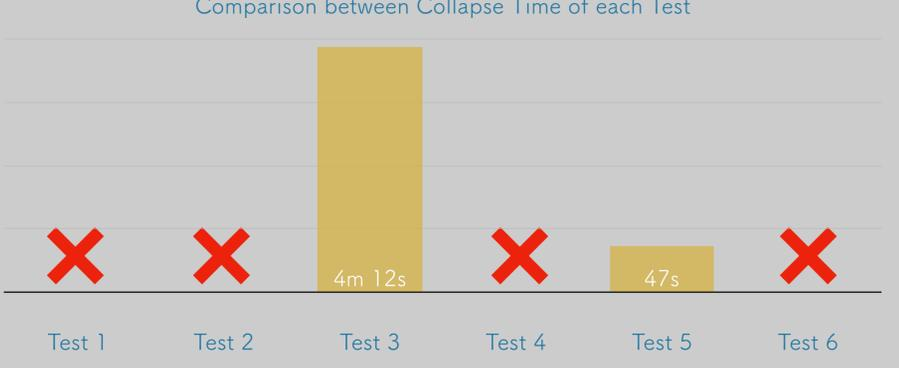
Test 3 (relative compaction 80%) and Test 5 (relative compaction 70%) collapsed. Indicating the soil is self-healing at these levels of compaction. Above 80%, it is not self-healing.
