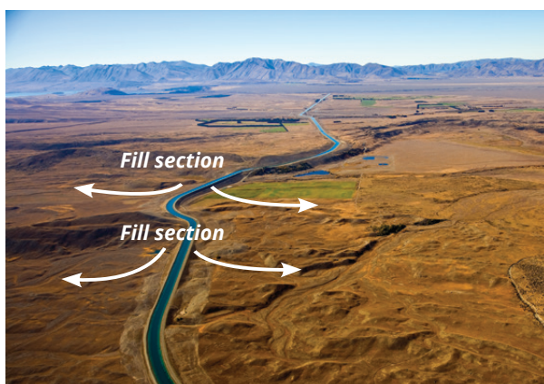
Figure 4.2: Example of canal 'fill' sections with different features and dam-break flow paths (provided by Meridian Energy)
